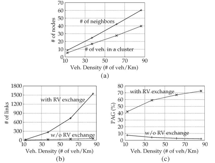
Fig. 6. Effect of range information exchange under ideal communication channels. (a) Number of nodes. (b) Number of available links. (c) Accuracy improvement.
