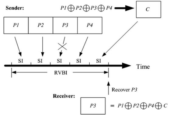
Fig. 18. Using coding in the RV exchange.
