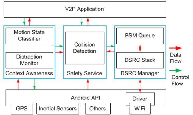
Fig. 1: V2P system design in smartphone
