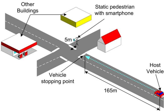
Fig. 7: LOS test setup
