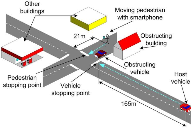
Fig. 6: NLOS test setup
