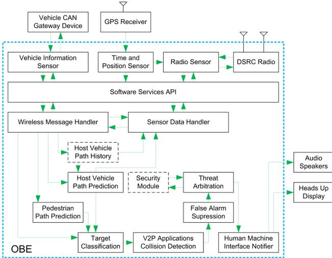
Fig. 4: V2P vehicle functional blocks
